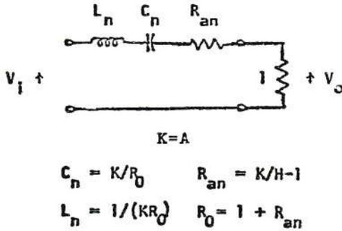
Fig. 7. First-order bandpass circuit and alignment formulas for the new crossovers. Calculate A, H parameters from first-order formulas in Table 5.
