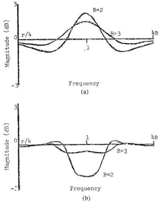
Fig. 2. Magnitude response of three-way crossover formed by parallel connection of two-way all-pass crossover filters. Here the bandpass is obtained by frequency transformation. Each graph shows responses for crossover frequency spreads of two ( $R = 2$ ) and three ( $R = 3$ ) octaves. (a) Second order. (b) Third order.
