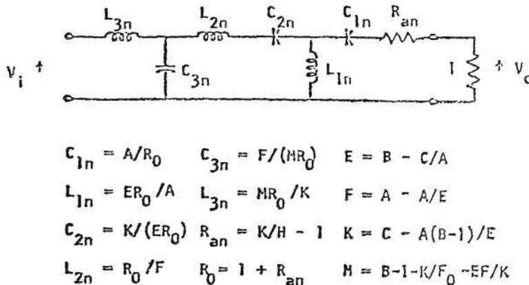
Fig. 9. Third-order bandpass circuits and alignment formulas for the new crossovers. Calculate A, B, C, H parameters from third-order formulas in Table 5.
