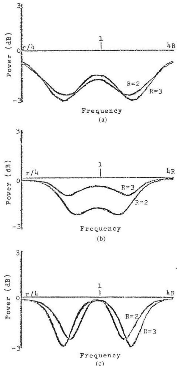
Fig. 4. Combined power response of the new three-way all-pass crossover networks. Each graph shows responses for crossover frequency spreads of two ( $R = 2$ ) and three ( $R = 3$ ) octaves. (a) Second order. (b) Third order. (c) Fourth order.
