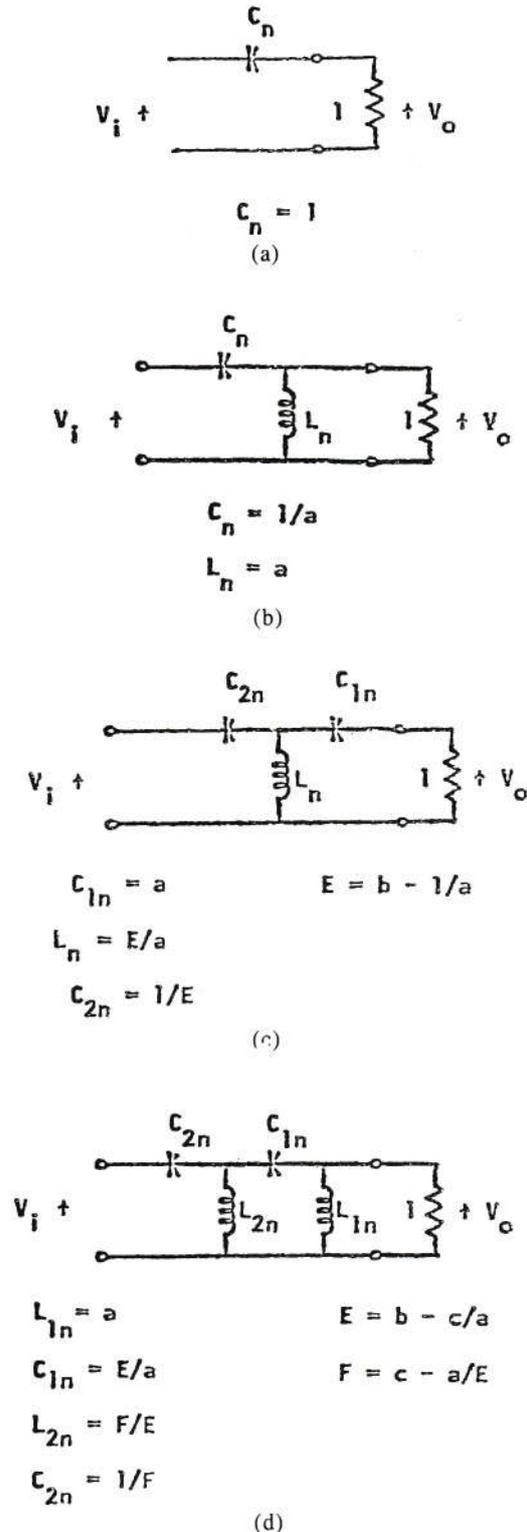
Fig. 6. High-pass filter circuits and alignment formulas for the new crossovers. (a) First order. (b) Second order. (c) Third order. (d) Fourth order. Relevant  $a, b, c$  parameters chosen as in Fig. 5.
