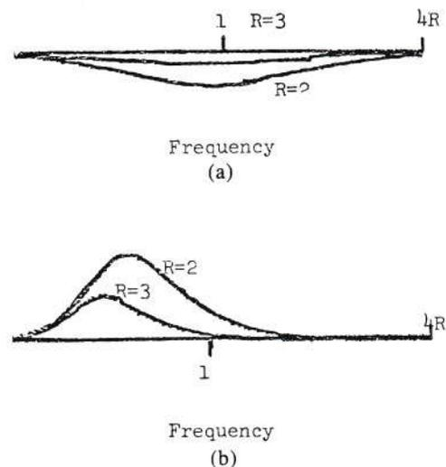
Fig. 1. Magnitude response of three-way crossover formed by cascading two-way all-pass crossovers. Each graph shows responses for crossover frequency spreads of two ( $R = 2$ ) and three ( $R = 3$ ) octaves. (a) Second order. (b) Third order.
