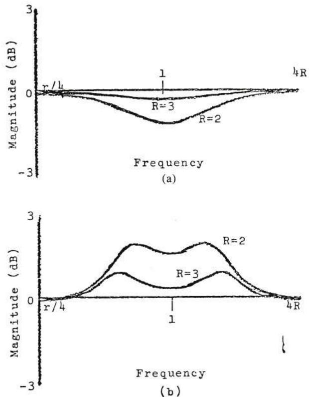
Fig. 3. Magnitude response of three-way crossover formed by parallel connection of two-way all-pass crossover filters. Here the bandpass is obtained by cascading. Each graph shows responses for crossover frequency spreads of two ( $R = 2$ ) and three ( $R = 3$ ) octaves. (a) Second order. (b) Third order.
