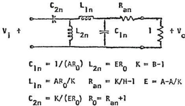
Fig. 8. Second-order bandpass circuits and alignment formulas for the new crossovers. Calculate A, B, H parameters from second-order formulas in Table 5.
