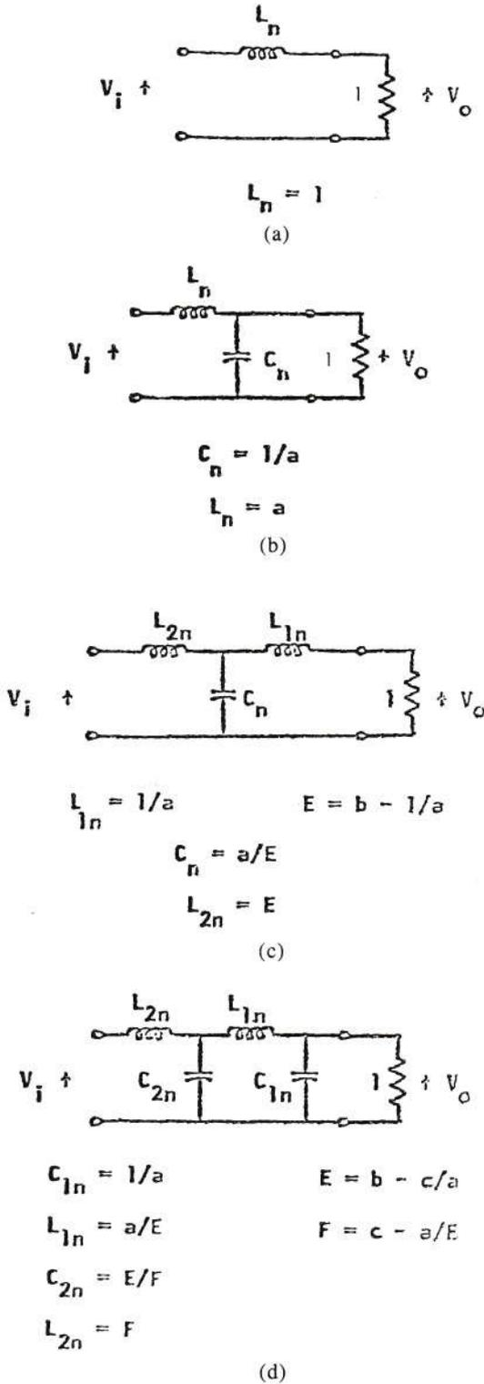
Fig. 5. Low-pass filter circuits and alignment formulas for the new crossovers. (a) First order, parameter  $a$  from Eq. (35). (b) Second order, parameters  $a, b$  from Table 2 or 3. (c) Third order, parameters  $a, b$  from Table 2 or 3. (d) Fourth order, parameters  $a, b, c$  from Table 4.
