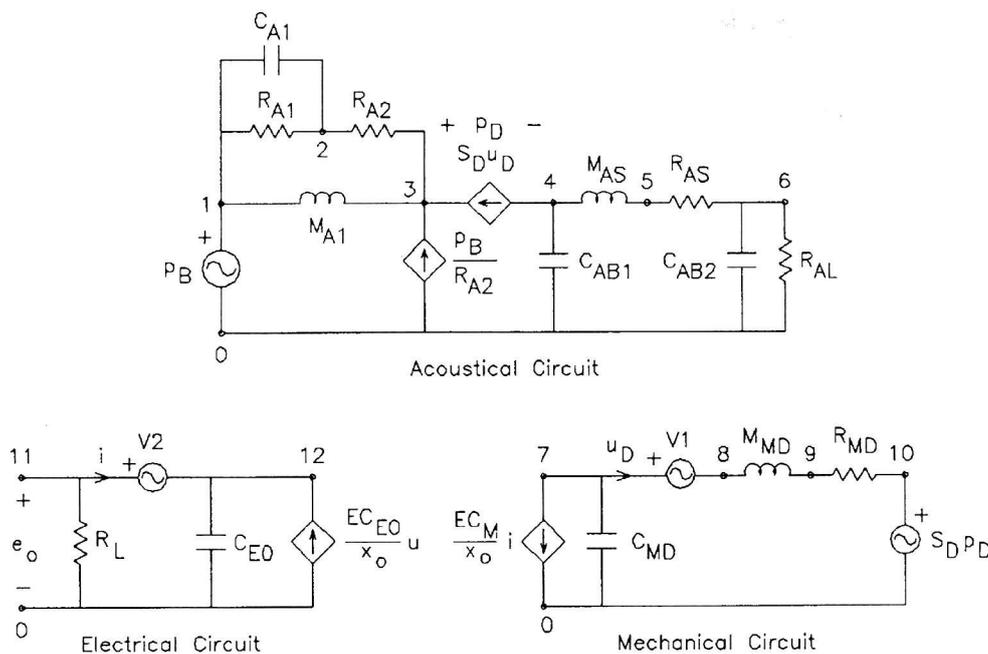
Fig. 12. Controlled-source analogous circuit for condenser microphone.
