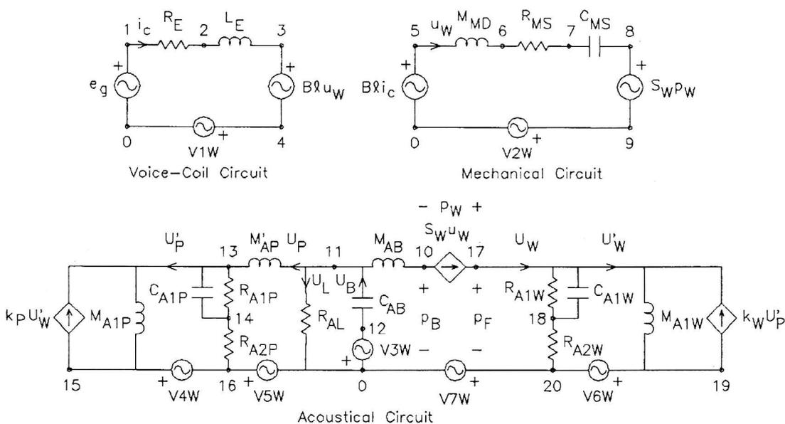
Fig. 9. Controlled-source analogous circuit for vented-box system.
