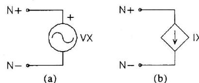
Fig. 1. (a) Constant-voltage source. (b) Constant-current source.
