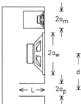
Fig. 8. Vented-box woofer and closed-box midrange.
