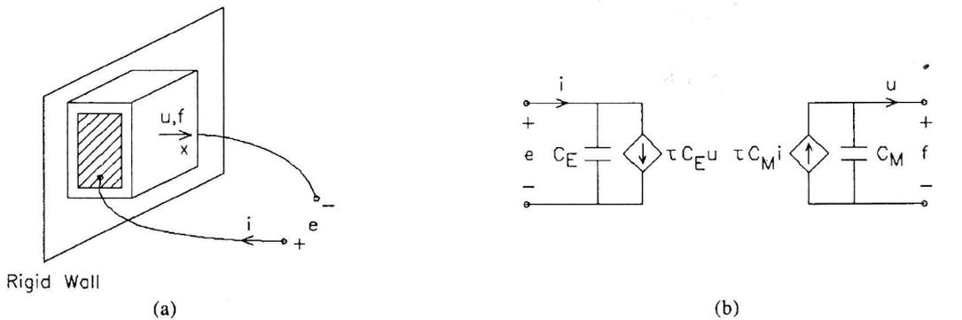
Fig. 3. (a) Crystal electrostatic-mechanical transducer. (b) Controlled-source model of transducer.
