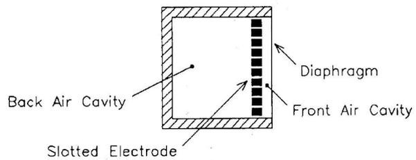
Fig. 11. Geometry for condenser microphone example.
