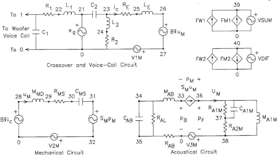
Fig. 14. Controlled-source analogous circuit for midrange and crossover networks.
