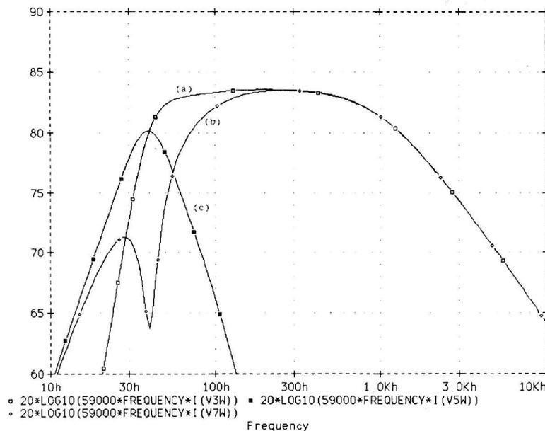
Fig. 10. Calculated on-axis SPLs at 1 m for vented-box woofer system. (a)—total system; (b)—woofer alone; (c)—port alone.
