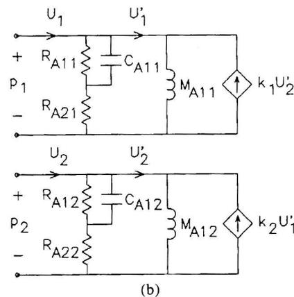
Fig. 7. (a) Mutual coupling between pistons in a common baffle. (b) Controlled-source analogous circuit for air loads on pistons, including effects of mutual coupling.
